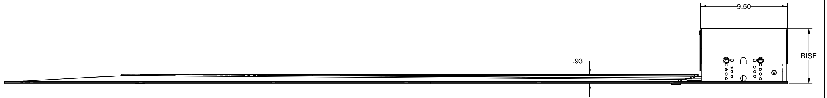
ELEVATION VIEW - STOWED POSITION (6" RISE SHOWN)
